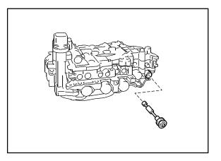
Repair Procedure (Continued)  b. Confirm that the manual valve lever is positioned as shown in the illustration and install the valve body assembly to the transaxle case with the 11 bolts.
