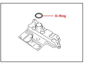
C. Remove the transmission valve body assembly.
