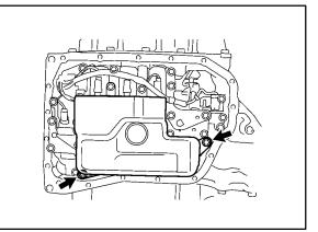
b. Remove the O-ring from the oil strainer.
