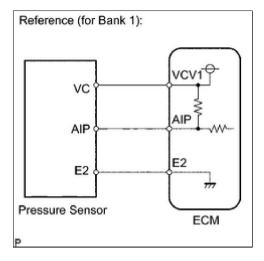
The ECM monitors the pressure in the secondary air passage using the pressure sensor located on the air switching valve in the secondary air injection system. Using this pressure value, the ECM determines whether the secondary air injection system is malfunctioning or not.
