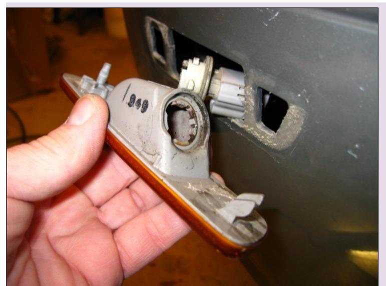
In this case the assembly was filled with water! The connector was also ruined - contacts eaten away. A lot of salt is used up here in the NE and everything rusts (if you noticed the undercarriage pics). I've ordered the crystal clear assemblies to replace and update from ProCarParts - \$36/pair + shipping (Dec 2003).
