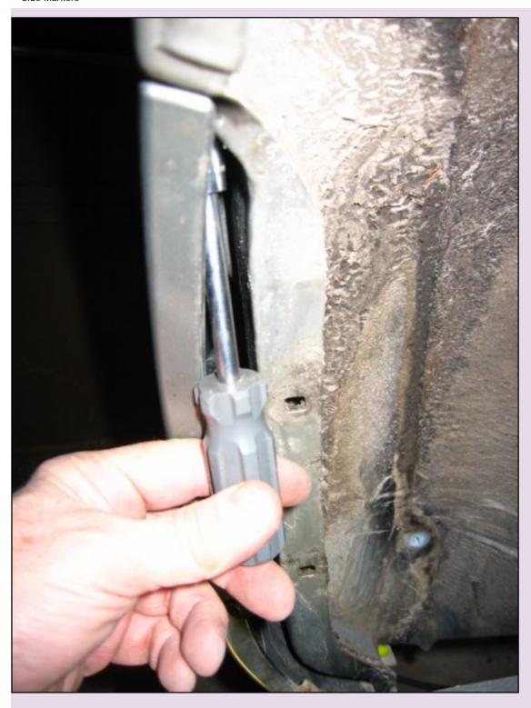
The best way to get to this bolt is with a long #3 Phillips screwdriver or nut driver (10mm) or a socket on a socket wrench with extension.
