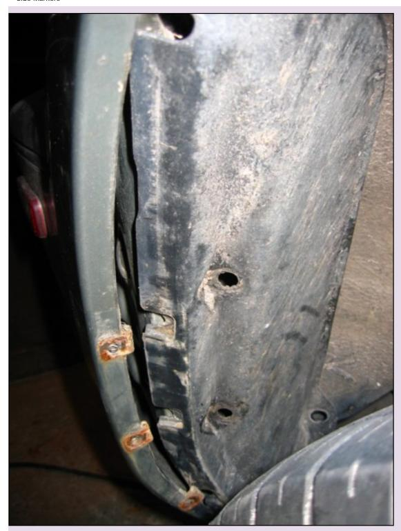
Once the inner shield is removed, there are 2 screws that must come out. The first is shown below at the front of the bumper cover below.
