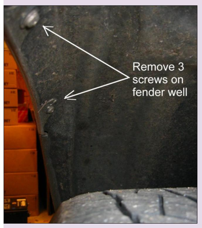
This is where the stubby Philips screw driver comes in handy (right). Of course jacking the vehicle several inches will help this and make easier for the whole job.
