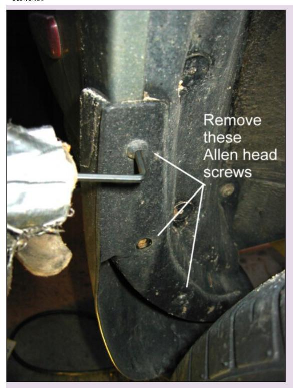
Next pry out the 2 plastic plugs in the inner plastic shield. These are difficult to pry out. Try not to break them, although mine almost came apart. If you break them, you may not need them for reassembly anyway. You have to remove one Philips screw (under the word "screws" in the above pic and behind the number "2" in the pic below).
