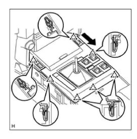
(c) Disconnect each connector and move the upper console panel in the direction of the arrow to remove it.
