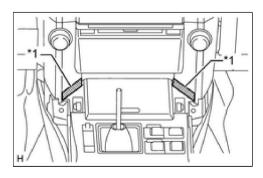
(a) Put protective tape around the upper console panel.
