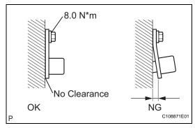
(a) Check the speed sensor installation.
