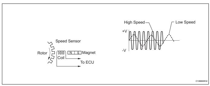
The speed sensor detects wheel speed and sends the appropriate signals to the ECU. These signals are used for control of the vehicle stability control system. The front and rear rotors each have 48 serrations.
