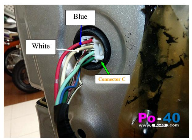
5. Connect the connector (**M9**) of harness to Po-40 main control unit and reassemble the door panel.
