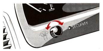
To adjust the brightness of the instrument panel lights, turn the knob with the headlight switch turned to the first or second clickstop.
