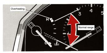
The gauge indicates the engine coolant temperature when the ignition switch is on. The engine operating temperature will vary with changes in weather and engine load.
