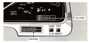
The odometer records the total distance the vehicle has been driven. The twin trip meter may be set to zero to record two different distances independently.
