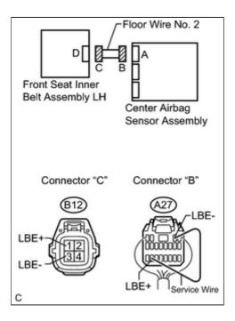
(b) Using a service wire, connect A27-19 (LBE+) and A27-2 (LBE-) of connector "B".
