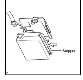
(a) Securely attach the rain sensor to the bracket.
