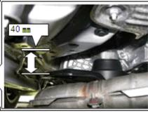
5. Support the T/M mount with a T/M Jack and lower T/M for 40mm.
