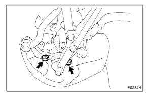
(c) Remove the 2 bolts and steering knuckle from the lower ball joint.
