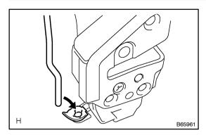
(c) Insert the door lock open rod into the door lock assy, and then set it to the door panel.
