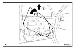
(c) Remove the door glass sub–assy, as shown in the illustration.
