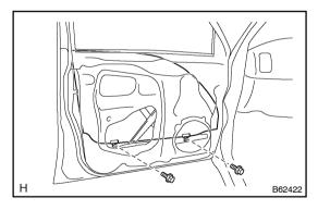
(c) Install the door glass sub-assy to the window regulator sub-assy with the 2 bolts.
