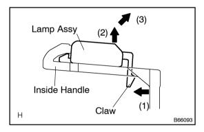
(k) Using a screwdriver, disengage the claw and remove the illumination lamp assy, as shown in the illustration.
