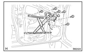
(b) Install the window regulator sub-assy with the 6 bolts.
