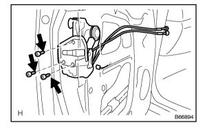
(d) Apply adhesive to the threads of the screws.
