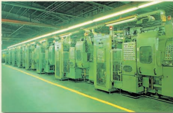
Grinding process of outer rings 外輪研削工程
