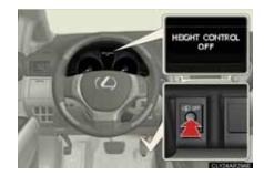
Press the height control off switch while the vehicle is stopped. A message will appear on the multi-information display, and vehicle height will be fixed in the current mode.
