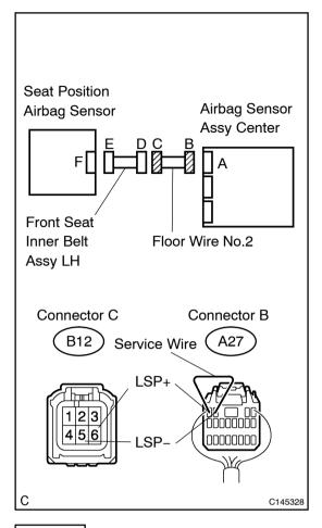
(a) Disconnect the front seat inner belt assy LH connector from the floor wire No.2 connector.
