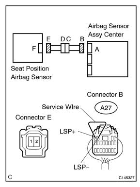
(a) Using a service wire, connect A27-4 (LSP+) and A27-3 (LSP-) of connector B.
